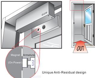
When the power is off, the holding force will be discontinuity and the bolt was installed in armature will pop out immediately. This design enables the door to be opened freely without any resistance.
