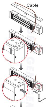
Fasten the mounting plate on the site then install electromagnet lock with power lead cable through mounting plate slot hole.
