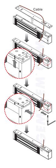
Fasten the mounting plate on the site then install electromagnet lock with power lead cable through mounting plate slothole.
