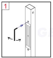
Use 3 mm hexagon tool wrench Use 4 mm hexagonal screw to operate the screw.
