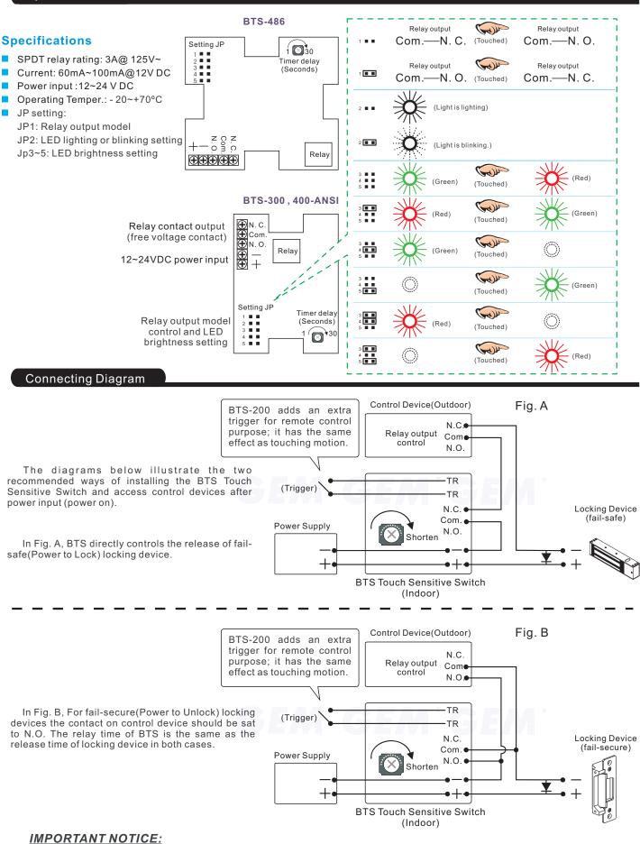
1. It is important to take extra notice on the maximum voltage and current output that the rated of relay contact to be used. 2. Make sure that the "+" and "-" wire are connected correctly.
