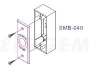
For the surface mount installation, the switch can be mounted with SMB-040 black plastic casing or SMB-040M for stainless steel housing.
