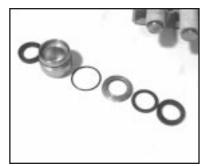
Remove the weep return ring (25), pressure ring (24), and v-sleeve (23) from the valve casing (26). Remove the v-sleeve (23) from the seal case (20).
