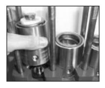
10. Place new plunger pipe (29B) carefully through the oiled seals and push seal sleeve (35) with plunger pipe into the crankcase guide. Note: Make sure weep hole is facing down.
