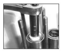
11. Tighten the tension screws (29C) to 310 in.-lbs. The plunger pipe (29B) should not be strained by over tightening of the tension screw (29C) or through damage to the front surface of the plunger; otherwise, it will probably break.
