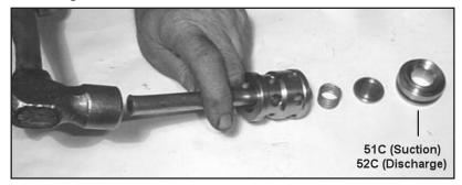
5) Valve seats (51C and 52C) are pressed out of spacer pipe (51F) by hitting the valve plate (51D) with a socket extention.
