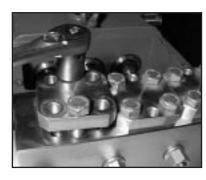
2) Take plugs (58) out of valve casing (50) by tightening screws (58C) against valve casing with two screws.
