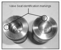
7) When reassembling: The inlet valve seat (51C) is 1mm smaller in diameter than the discharge valve seat (52C). Inlet valve seats are marked "S" and always have to be installed first. Discharge valve seats are marked "P" and are always to be installed on top of inlet valve. Plugs (58) are to be tensioned down evenly with screws (58C) and in crosswise pattern at 155 (ft.lbs.).
