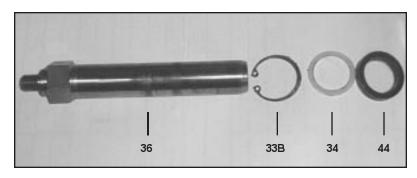
17) Examine plunger (36) for signs of wear or cavitation. If the surface of the plunger is worn, screw out the plunger with a 27mm tool. Clean centering and front surface of crosshead with plunger (25). Thread new plunger carefully through oiled seals in seal sleave. Coat thread of new plunger lightly with bonding agent (e.g., loctite).
