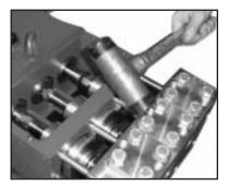
9) With a rubber mallet tap the back of the valve casing (50) and pull the valve casing off the stud bolt (49).
