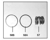
3) Remove the compression spring (57) O-Ring (58A) and support ring (58B).
