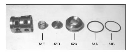
6) Check surfaces of valve plate (51D), valve seat (51C or 52C), o-rings (51A), and support rings (51B). Replace worn parts.
