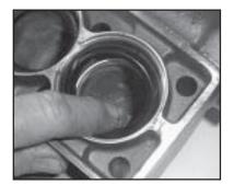
10. Place support ring (41) and v-sleeves (40) into valve casing.
