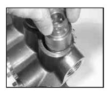
38. Reassemble the inlet valve assembly in the reverse order of step #7. Make certain all the components are press fit together and that the spring retainer (#54) is slightly counter sunk in the valve housing (#52). Grease the o-ring (#53) and install it on to the valve housing. Reinstall the entire inlet valve assembly into the manifold (#43). install the tension plugs (#42A) and tighten.
