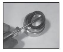
8) Remove the weep grooved seal (23 or 23B) together with pressure ring (24 \_ P420 and P425 only) out of the seal adaptor (20). Check O-rings (21).
