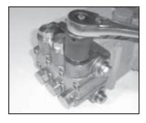
1) With a socket wrench, remove the three discharge valve plugs and three inlet valve plugs (32). Inspect the o-ring (33) for wear and replace if damaged.
