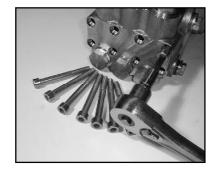
5) Use a 8mm allen wrench to remove the 8 socket head cap screws (34). Carefully slide the valve casing (26) out over the plungers. Remove the weep return rings (25).
