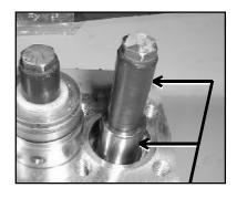
9) Check surfaces of plunger pipe (16B).
