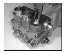
2) Using needle nose pliers, remove the inlet and discharge valve assemblies (27A). Note: It may become neccesary to remove the valve seat (27) from the valve casing using a slidehammer.
