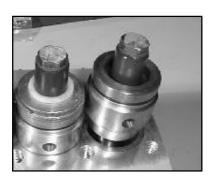
10) Place each seal case (20) with new o-rings (21 and 22) and new oil seals (19) over plungers (16) with weep hole down. Generously lubricate o-rings and oil seals before reassembly.
