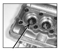
13) Generously lubricate v-sleeves. Assemble spacer rings (23A), and v-sleeves (23) into valve casing (26).
