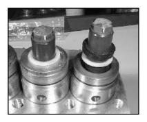
11) Place pressure rings and weep seals (23B) over plungers and into each seal case (20).
