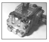
2. Using a needle nose pliers, remove the inlet and discharge valve assemblies (27-31).
