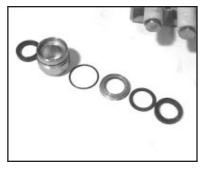
7. Remove the weep return ring (25), pressure ring (24), and v-sleeve (23) from the valve casing (26). The spacer ring (30A) on CP230 pumps may remain inside the valve casing.
