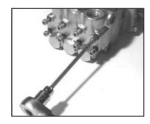
5. Next, use a 5mm allen wrench to remove the 8 socket head cap screws (34).
