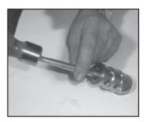
3. Valve seats (51C and 52C) are pressed out of spacer pipe (51F) by hitting the valve plate (51D) with a bolt.
