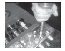
2. Take out complete valve assemblies (51 and 52) using either tool (part #07662) or stud bolt.
