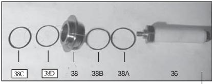
10. If o-rings (38A and 38C) or support rings (38B and 38D) are damaged, replace with new parts. Examine plunger (36) for wear.
