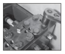
1. Lossen screws (58C), take plugs (58) out of valve casing with two screws.
