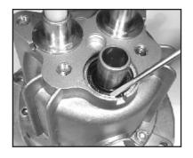
12. If the crankcase oil seals (15) are to be replaced, they can be removed by prying loose with a screwdriver. Take care not to make contact with the plunger (8) and pry out the oil seals from their housing. Seals should not be reinstalled until after step #16.
