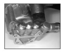
10. Tap the back of the manifold (35) with a rubber mallet to dislodge, and slide off the plungers. (8). Take note of the position of the discharge port so as to place the manifold in the same position during reassembly.
