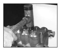
15. Place entire manifold/seal sleeve assembly over the studs and push firmly until seated
