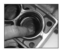
13. For LP255 pumps, insert support ring (37) into valve casing (43). Place support ring (41) and v-sleeves (40) into valve casing.
