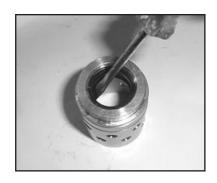
The front oil seal (31A) can now be removed by inserting a screwdriver through the rear of the retainer and tapping the seal out through the front of the retainer. Remove any excess old loc-tite from retainer. To replace oil seal, apply a light film of loc-tite around outside edges of seal. Tap seal firmly into the retainer with a wooden dowel making certain that the spring side of the seal is installed first and that the seal sits squarely in the retainer.
