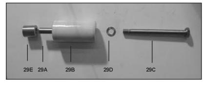
6. Inspect surface of plunger pipe (29B) carefully. Remove any chemical or mineral deposits taking care not to damage the surface of the plunger. If plunger pipe is worn, remove the plunger bolt (29C), plunger pipe (29B) and spacer (29E). Replace worn parts necessary. Note: Always use a new copper gasket (29) when repairing the plunger assembly.
