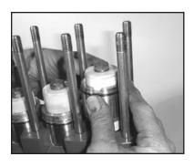
7. For LP122A & LP122A-4000 pumps, oil seal replacement can be accomplished by pulling the retainer forward out of the crankcase. The o-ring around the outside of the retainer should be replaced and lubricated with a light film of
