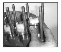
14. Press seal sleeve assembly into the manifold and seat firmly. Put the support ring (41) on plunger with v-side facing the manifold.
