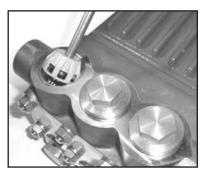
17. Next, place valve assemblies (46A) into manifold after first lubricating the o-ring (44A). Seat
