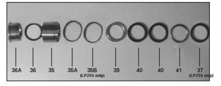
4. Remove the seal sleeve (35) from the manifold and/or crank-case. Remove the pressure rings (39&36A), v-sleeves (40&36), support ring (41) and o-rings (35A and 35B in Lp255A only) from the manifold and seal sleeve, respectively. For LP255 only, remove support ring (37). Examine seals carefully and replace if worn. Clean all parts.
