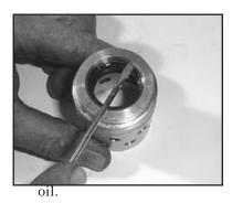
8. The back-up seal (33) can be pried out of the back of the retainer (32) with a small screwdriver. To replace with new seal, lubricate edges of new seal, then squeeze outside edges of seal, forcing the seal to collapse into a figure 8. Tuck the two outside edges of the figure 8 into the rear of the retainer, making sure that the inner lip of the seal faces the oil. The seal may now be pressed firmly into place.
