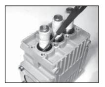
9. If the crankcase oil seals (19) are to be replaced, they can be removed by prying loose with a flat screwdriver. Take care not to make contact with the plunger.
