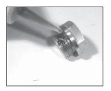
4. Remove the o-ring (31). Inspect all parts for wear and replace as necessary. Apply one drop of Loctite 243 to the valve plugs (32) and tighten to 59 ft.-lbs.
