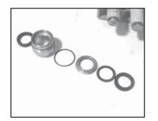
Remove the weep return ring (25), pressure ring (24), and v-sleeve (23) from the valve casing (26). Remove the v-sleeve (23A) from the seal case (20). Inspect all parts, including o-ring (21) for wear and replace as necessary
