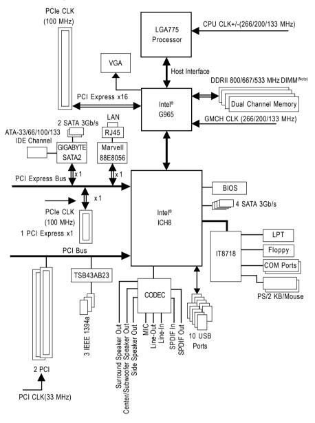
(Note) To use a DDR II 800/667 memory module on the motherboard, you must install an 1066/ 800 MHz FSB processor.
