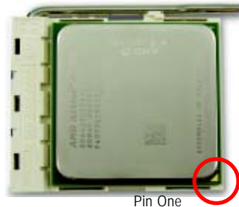
Fig.2 Pin 1 location on the socket and CPU. Gently place the CPU into position and make sure the CPU pins fit perfectly into the holes. Once the CPU is positioned into its socket, place one finger down on the middle of the CPU and gently press the metal lever back into its original position.
