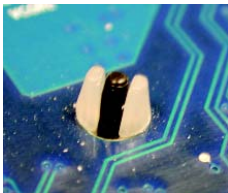
Fig. 5 Please check the back of motherboard after installing. If the push pin is inserted as the picture, the installation is complete.
