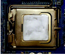
Fig. 1 Please apply an even layer of CPU cooler paste on the surface of the installed CPU.
