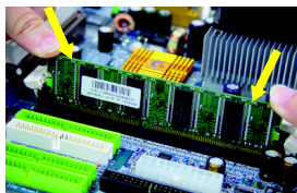
Fig.1 The DIMM socket has a notch, so the DIMM memory module can only fit in one direction. Insert the DIMM memory module vertically into the DIMM socket. Then push it down.
