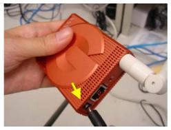
Step2 Connect one end of the Ethernet cable to the LAN port of the Game Adapter.
