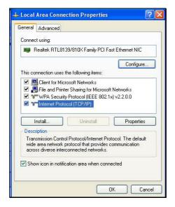
Step 5. Assign the static IP address used by the AP and the same Subnet Mask to the computer (For example, IP address is192.168.1.2 and Subnet Mask is 255.255.255.0), click the "OK" button to return to "Local Area Connection Properties". Click the "OK" button again to complete the PC configuration.
