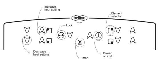
When the hob is first switched the controller will illuminate parts of its displays. accompanied by a beep. This is the controller testing and calibrating itself. When this process is complete the neon adjacent to the lock pad will light, to indicate the hob is ready for use but locked for safety.
