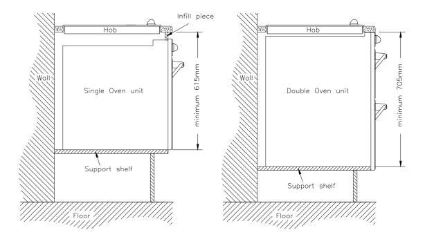
The hob can be fitted above a Belling built-under single or double
