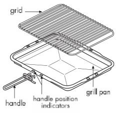
Place the handle over the edge of the grill pan, at the narrow side edges. Slide the handle to the centre, and locate between the handle position indicators.
