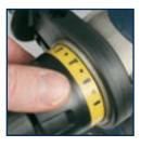
For drilling, always use the use the Drill position by aligning the Drill symbol with the triangular indicator on the front face of the drill near the torque collar.
