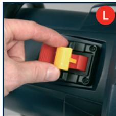
2. Lift the switch to the ON position (I) to turn on and operate the dust collector (fig. M).
