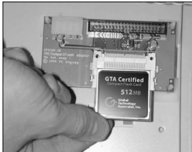
Inserting the Compact Flash Card into the IDE Adapter Board
