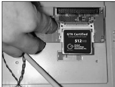
Mounting the Compact Flash IDE Adapter Inside the Intended Firewall
