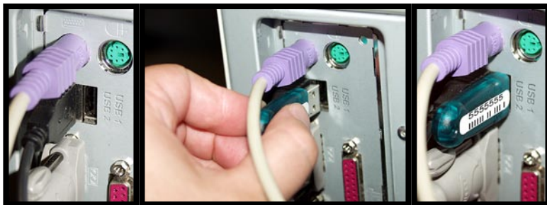
Installation of the USB Key Block
