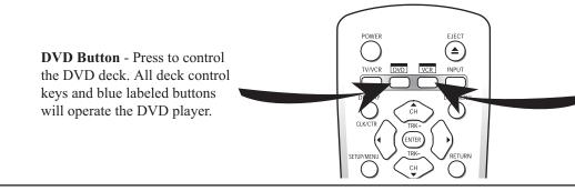
VCR Button - Press to control the VCR deck. All deck control keys and red labeled buttons will operate the VCR.
