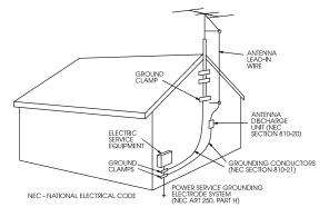
provides information with regard to proper grounding of the mast and supporting structure, grounding of the lead-in wire to an antenna discharge unit, size of grounding conductors, location of antenna-discharge unit, connection to grounding electrodes, and requirements for the grounding electrode. See figure above.
