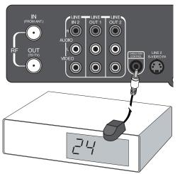
Position the Cable Mouse directly over the IR (infrared) remote sensor.
