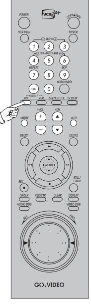
Pressing the TV key puts the remote control in TV mode. Some or all of the highlighted keys will be able to control your television.
