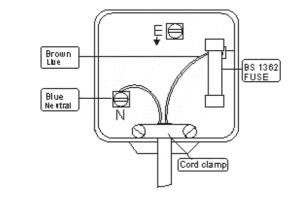
The wires in this mains lead are coloured in accordance with the following wiring codes:
