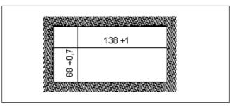
The paper reroll mechanism is inserted into the DIN size panel cutout from the front side and is clamped against the rear of the switchboard using the mounting screws. The switchboard thickness must not exceed 12 mm.
