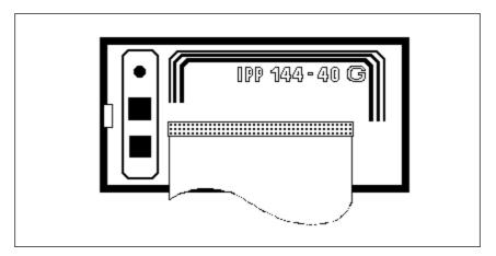
The Thermal Graphics Printer IPP 144-40 G (Industrial Process Printer) is a device designed for outputting text, data and graphics, i.e. measured value, machine and process states, error messages, production data, etc.
