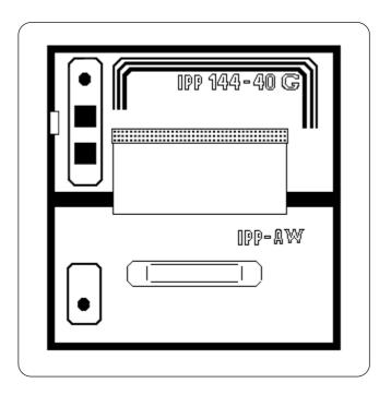
The IPP-AW is a paper reroll mechanism designed for use with the Thermal Graphics Printer IPP 144-40 G. It has been designed to match the printer in colour and style. It is preferably installed directly underneath the printer. The printed paper is automatically wound on a drum by a motor. A front panel draw allows easy paper handling.
