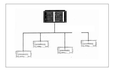
Each printer is addressable, which allows the connection of up to 31 devices to one sender device via a data line at the RS 485 interface, e.g. to a PLC.
