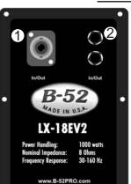
The LX-18EV2 includes (2) 1/4" phone jacks and one Neutrik NL4 Speakon input terminals. All three terminals are internally connected in parallel. Each of the three connections can be used as an input or as an output.
