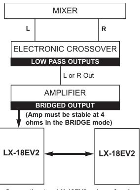
Connecting two LX-18EV2 subwoofers in parallel results in a 4 ohm load.
