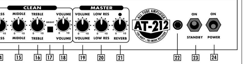
frequencies as desired in the clean channel. Turning the middle control clockwise will increase the amount of warmth in your tone. Counterclockwise settings create a more pristine, acoustic kind of sound.
