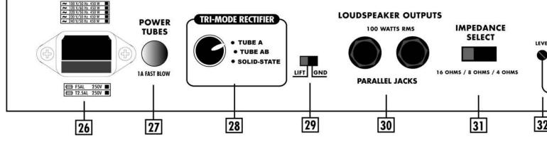
26. AC INLET & PRIMARY FUSE: Connects AC powercord and houses primary fuse.
