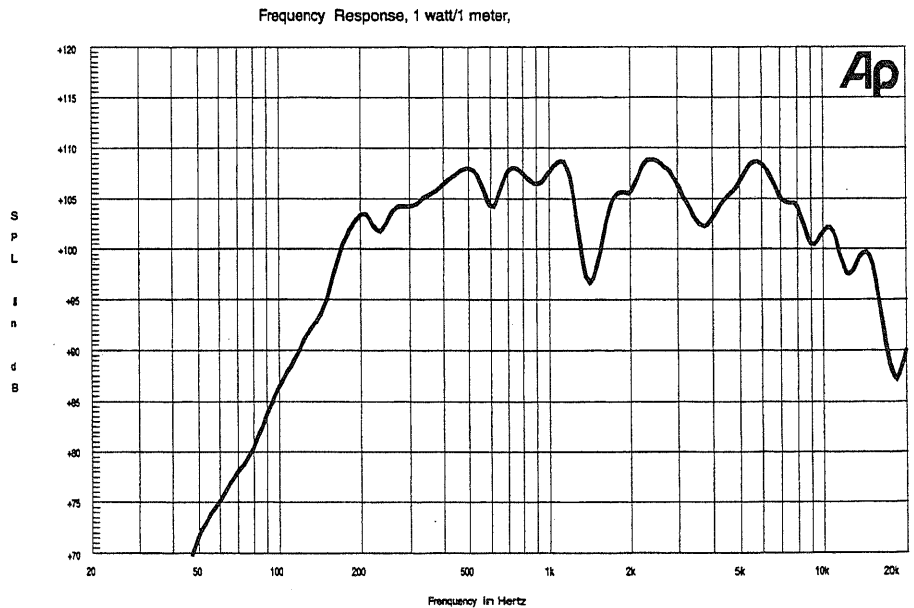
Figure 4—Axial Frequency Response (anechoic environment, 1 watt/1 meter into mid-bass section)
