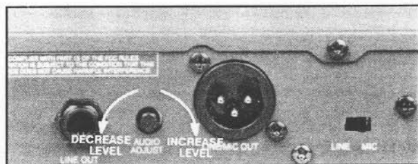
Figure 3 - Adjust Audio Output Level, Rear Panel
