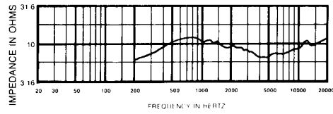
FIGURE 6 — Impedance Response, 2-Inch Plane-Wave Tube, 8-Ohm Driver
