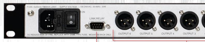
RS-232 port for Master/Slave connections or GPI preset recall
