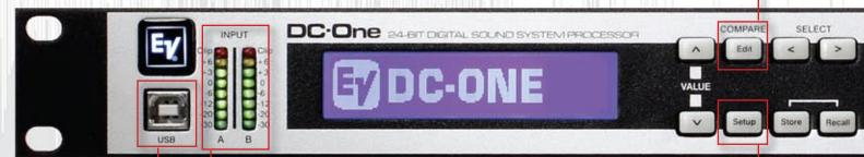
Reliable, accurate input metering assures proper gain staging.
