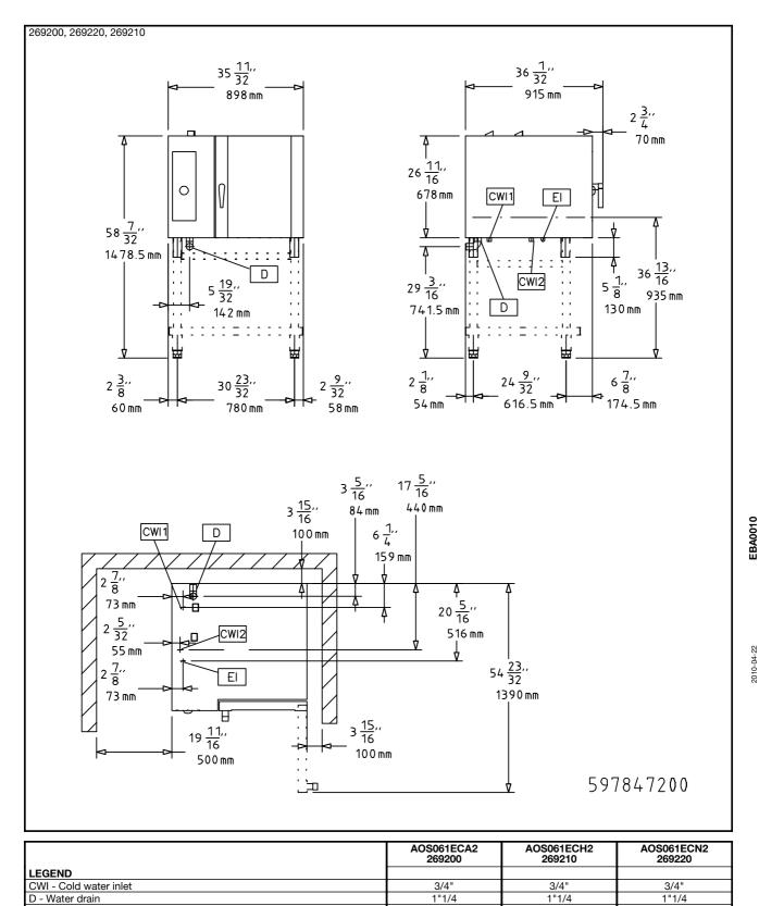
EI - Electrical connection WIC - Cooling water inlet 400 V, 3N, 50/60
