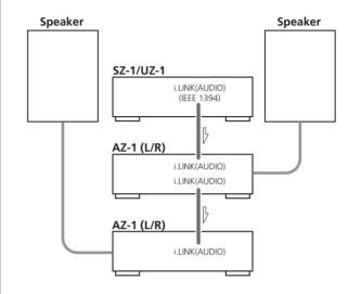
The MASTR and SLAVE settings of the i.LINK remote control function allow you to set one AZ-1 as master and the other as slave, so that the volume, muting and dimmer of the two AZ-1's can be controlled in unison using one of the pair units.
