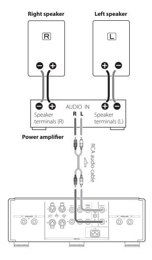
Connect the PRE OUT terminals to the analog audio input terminals of the power amplifier using commercially available RCA audio cables.
