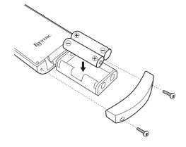
Use a Philips screwdriver to remove the cover from the bottom of the remote control, and slowly pull out the battery case. Insert two AA batteries in the correct  $\oplus/\ominus$  orientations, reinsert the case and close the cover.
