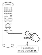
"Disp>" appears on the display and the unit enters the setup mode.
