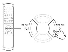
Each time the INPUT buttons (</>) is pressed, the available terminal names changes as follows:
