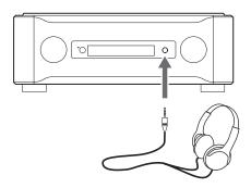
For private listening, insert a 6.35~mm (1/4'') stereo headphone plug into the PHONES jack, and then adjust the volume by turning the VOLUME knob.
