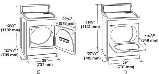
\*Most installations require a minimum 5" (127 mm) clearance behind the dryer for exhaust vent with elbow.
