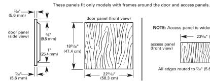
NOTE: Access panel is wider than door panel. 235/16" (59.2 cm) access panel (front view) All edges routed to 7/32" (5.6 mm) thickness
