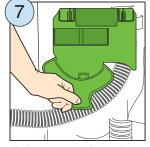
Pull out bottom of lower hose retainer and position hose.
