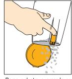
Remove dust cup; press lever to release bottom lid.
