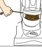
Pull out cord to desired length. Do not pull past red line; push cord into cord clip.
