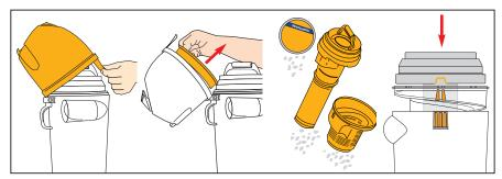
Pull filter latch to release cover. Lift out foam filter and shake off dust. Lift out filter tube with screen; shake off dust. Reinstall filters and close cover.
