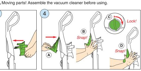
Insert top tab A turbo holder into handle. Place thumbs on each side and snap bottom corners **B** into place. Turn **C** knob to lock. Store turbo nozzle in holder. Some models: Snap D turbo cover straight on from front to back.
