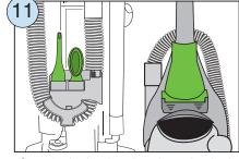
Store dusting brush and crevice tool on back of vacuum. Store turbo nozzle in holder (tools vary by model).
