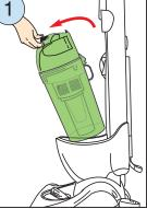
Remove dust cup to assemble vacuum.
