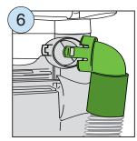
To install hose connector, align tab at right and snap on at left.
