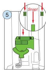
Place lower hose retainer in slots on back of vacuum. Push down to snap into place.
