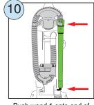
Push wand 1 onto end of hose. Place over bottom hook; snap in at top.
