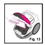
Knock the dust of the motor protection input filter (11) thoroughly or wash it if it is very dirty, making sure that it is completely dry before refitting. Never use the vacuum cleaner without the motor protection input filter.
