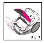
• Push back the black plastic tabs (A) towards you. This will release the cardboard base of the dust bag from the hooks (B), and allow you to slide the full bag upwards. (See fig. 8)
