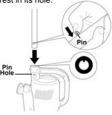
• To insert the upper piece of the metal handle, press on the pin that is on the upper handle and insert into the lower handle making sure that the pin comes out of the pinhole on the lower handle.
