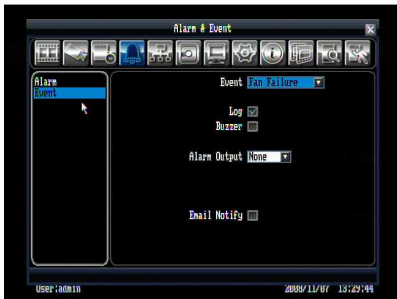
Figure 5.13 (Alarm & Event Menu – Event-Fan Failure)
