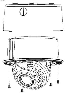
6. Screw the 2 spring tabs *in the orientation shown* to the slots at both sides of the inner base using the 4 Philips head screws provided. Attach the screws to the places marked "Fix".
