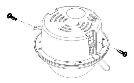
7. Attach power and video cables from source to cables from camera and push excess wire back into hole. Fold the spring tabs up.
