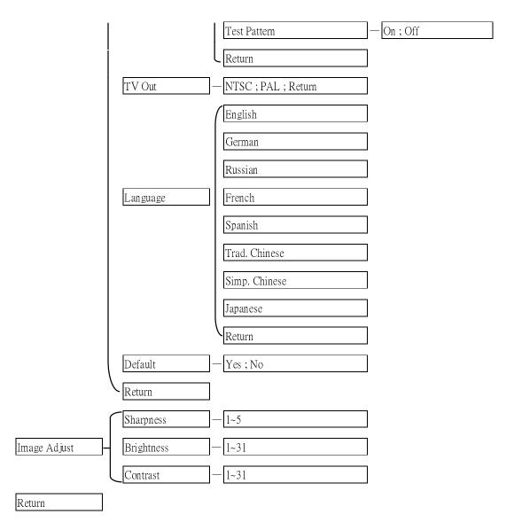
Press Set button to enter SETUP Menu. In SETUP menu, use the joystick to make settings. User can do camera settings including Exposure, White balance, Day/Night, Special and Image adjust. Please select the item by moving the joystick UP or DOWN then press SET to enter the settings. Move the joystick to the last option which is "Return" to return to live view.
