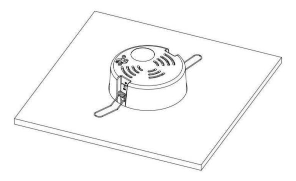
11. Use the long Phillips pan head screws (x4) provided to screw the base to the ceiling. Do NOT use washers.
