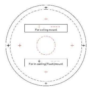
2. Use the appropriate tool to drill the OUTER holes; carefully cut along the dashed circle to create a clearance hole for the inner base unit.
