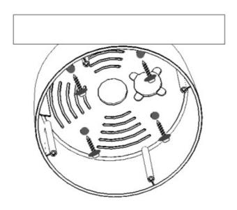
7. Attach power and video cables from source to cables from camera and push excess wire back into hole.
