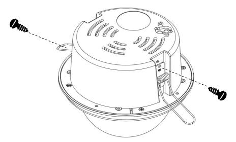
7. Attach power and video cables from source to cables from camera and push excess wire back into hole. Fold the spring tabs up.
