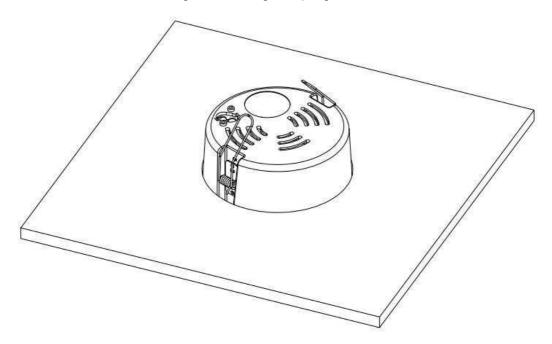
10. The spring tabs will open automatically to support the camera against the ceiling.
